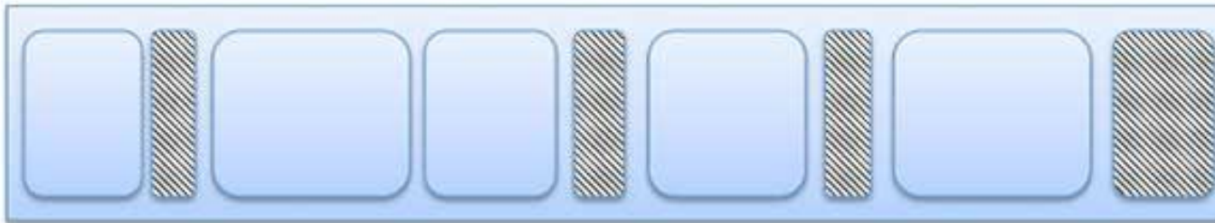
Fragmented memory before compaction
